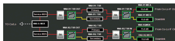
Example: Protection Switching Dashboard where two sources and two sets of equipment are switched out to a single destination.
