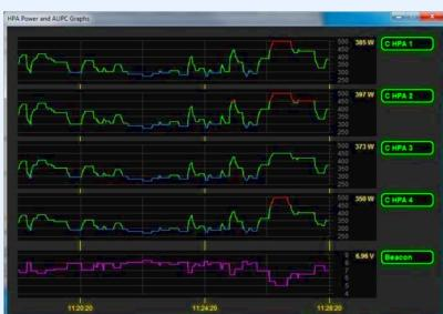
The Uplink Dashboard makes it easy for operators to know if they are transmitting the right amount of power to each transponder. This dashboard displays:
